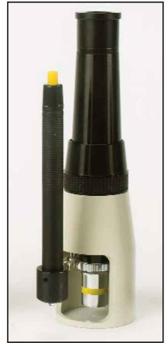
Microscope shown with standard torch accessory
